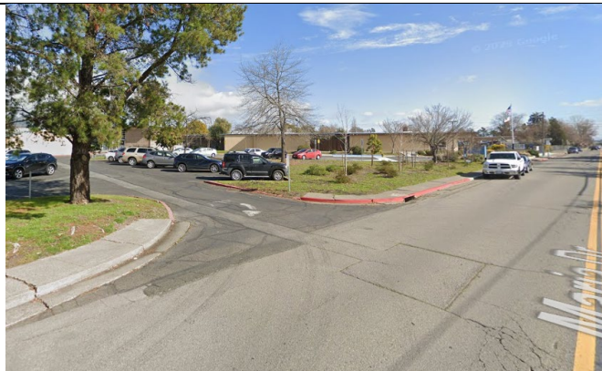
Loma Vista driveways (Install accessible curb ramps, remove two parking spaces between driveways and install bike lane along full length of red curb)
